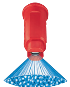
Figure 7. Flat fan nozzle spray pattern.
