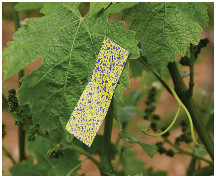
Figure 9. A water sensitive card after the spraying is finished. This pattern on the card represents ideal coverage for the target being sprayed.
