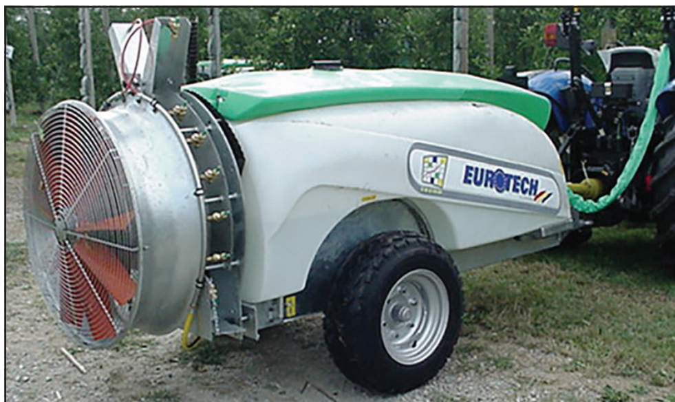
Figure 3. A typical airblast sprayer used in orchards and vineyards in U.S.
