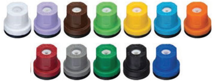
Figure 10. One-piece, color-coded, hollow-cone nozzles, each of which have their own flow rate. Flow rates increase from 0.053 gal/min (the white nozzle on the left, with the smallest orifice) to 0.49 gal/min (the blue nozzle on the right with the largest orifice) at the rated spray pressure of 40 psi.
