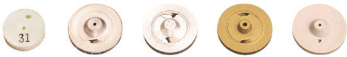
Figure 7. Cores with slanted holes that are used in disc-core nozzles to spray a cone pattern. The four cores with a hole in the center of the plate spray a full-cone pattern. The core in the middle without a hole in the center of the plate sprays a hollow-cone pattern.
