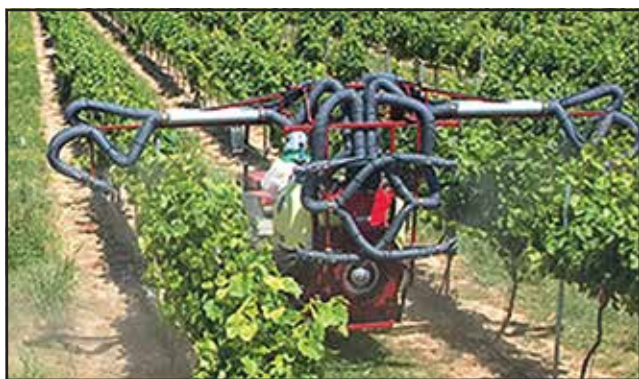
Figure 31. Sprayer covering both sides of two rows of grapevine in one pass.
