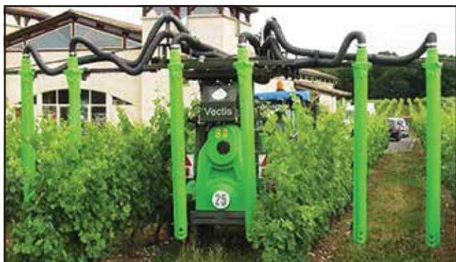
Figure 33 (left). Sprayer with two vertical manifolds per row. Each manifold has air spouts and nozzles on one side which allows each manifold to only spray one side of the row.
