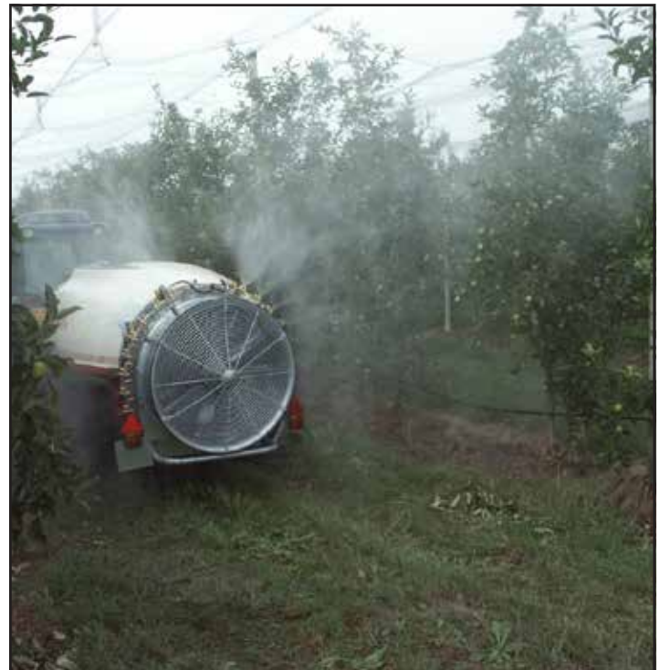
Figure 8. Airblast sprayer with no deflector plates. The top nozzles are turned off—a desirable practice.
