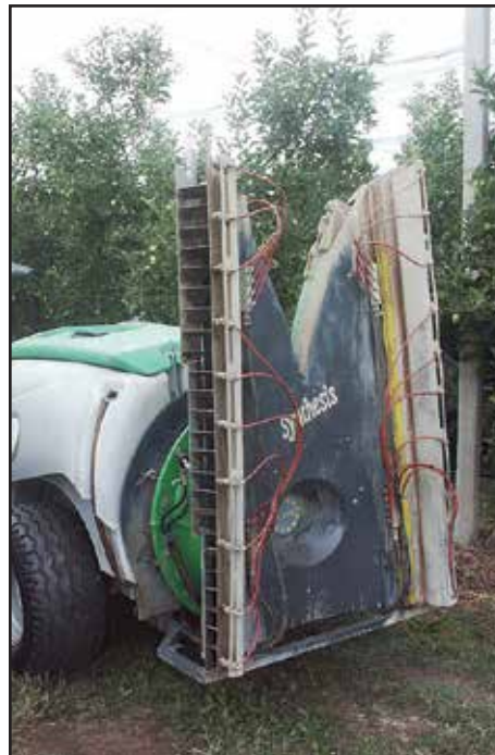
Figure 17. Tower sprayer with three different sizes of air exit ports. Notice the seven ports near the ground have the smallest cross section allowing less air to be discharged, while the top eight ports have the widest cross section allowing more air to be discharged from the top part of the shroud.
