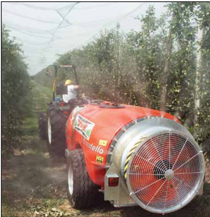
Figure 7. Airblast sprayer with no deflector plates. Notice the top three nozzles should have been turned off because they are not directed towards the target.
