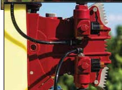
Figure 28 (above). Tower sprayer with adjustable air ducts and with two nozzles per spout.
