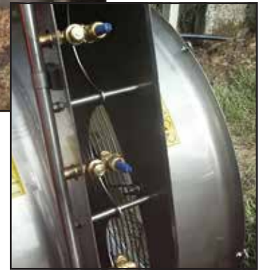
Figure 15 (below). Close up of the vertical air shroud with internal deflector plates for uniform distribution of the air from top to bottom of the air delivery shroud.
