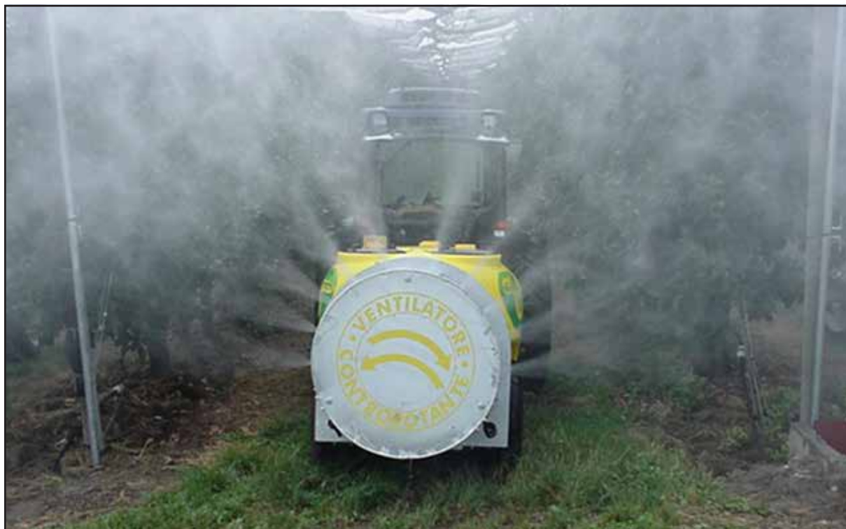
Figure 11. Airblast sprayer with adjustable deflectors. Notice the nozzles on this sprayer are located inside the air outlet port of the fan.
