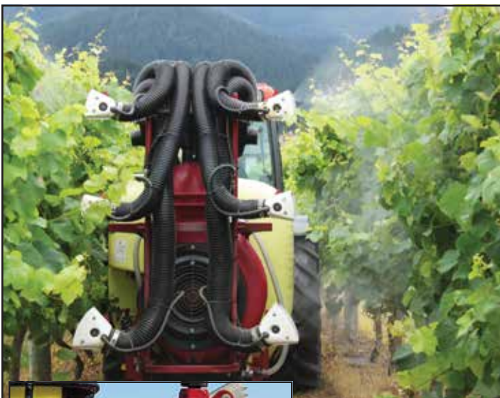
Figure 28 (above). Tower sprayer with adjustable air ducts and with two nozzles per spout.
