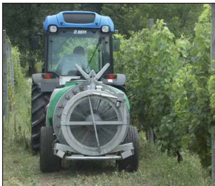
Figure 13. This rear view of the airblast sprayer shows the deflectors properly adjusted according to the canopy height.
