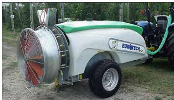
Figure 11. Airblast sprayer with adjustable deflectors. Notice the nozzles on this sprayer are located inside the air outlet port of the fan.
