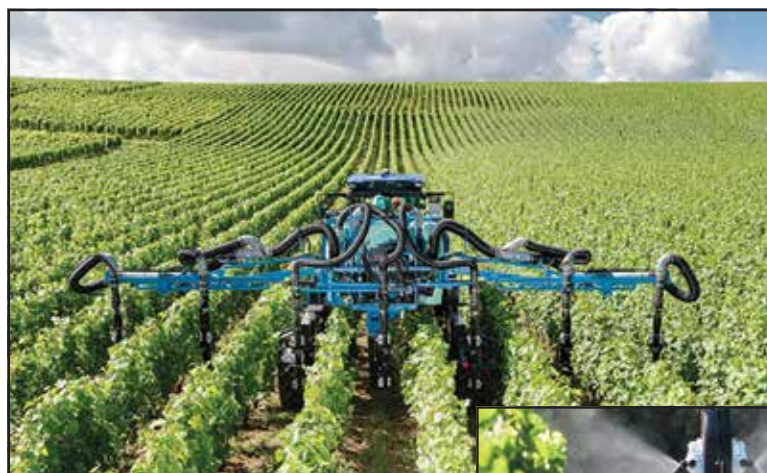
Figure 32a. Sprayer with single vertical manifolds between rows with air spouts and nozzles on both sides spraying multiple canopy rows.
