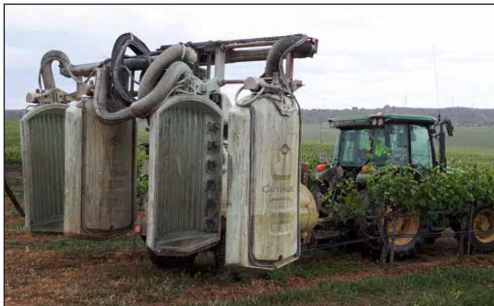
Figure 37. A two-row tunnel sprayer with excess spray recirculation system.
