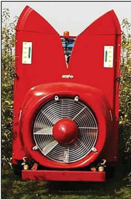
Figure 16. Close up of the vertical air shroud with internal deflector plates for uniform distribution of the air from top to bottom of the air delivery shroud.
