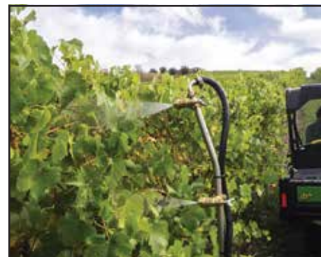
Figure 5. Close-up of vertical boom with two adjustable-flow nozzles spraying the vineyard canopy.
