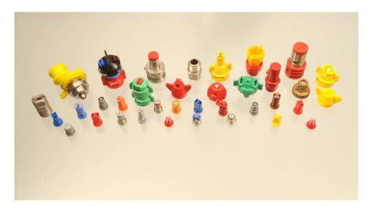
Generally, in forestry applications, even flat-fan spray nozzles are most desirable for band or spot spraying. They provide the most even distribution of spray material over the area treated. Sprayers must be calibrated for each nozzle type and size.
