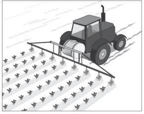
With the sprayer stationary, and the operating pressure set to the same pressure that will be used in the field, place a measuring cup with a capacity of at least 1 quart
