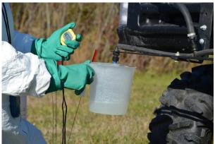
Determine the Volume of Spray Delivered by Nozzles Single Nozzle Per Band
