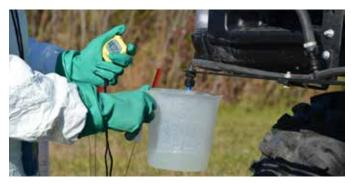
Determine the Volume of Spray Delivered by Nozzles
