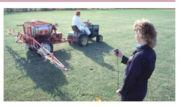
is actually sprayed. Many different configurations and types of tractor-drawn sprayers can be used to spray herbicides in bands including: fixed boom with one or more nozzles; hose and spray gun operated by a person walking; and a hose with small handheld booms.
