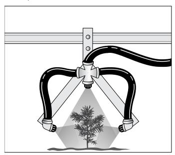
If multiple nozzles are used to spray a single row, determine the delivery rate of each nozzle in GPM as explained above, and add the amounts together to obtain the total amount of spray in GPM being delivered to the row.
